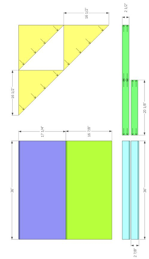
Drill pocket holes for 1-1/4" pocket hole screws as indicated by the arrows. All of the face frame pieces are ripped from a piece of 1 × 6.
